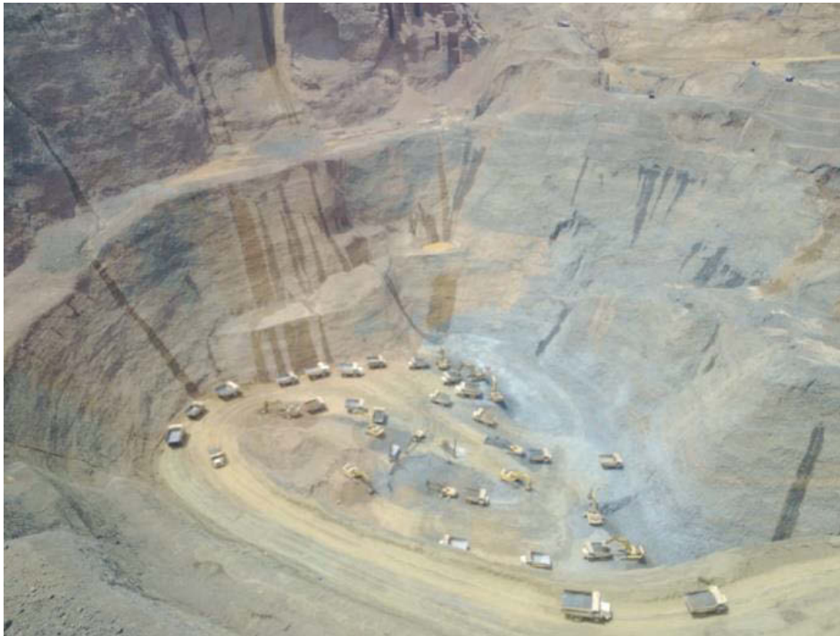
Plate 3.1 Large-scale mining to expose deep Uru Boulder Conglomerate
